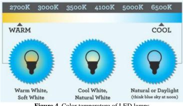
Figure 4. Color temperature of LED lamps
